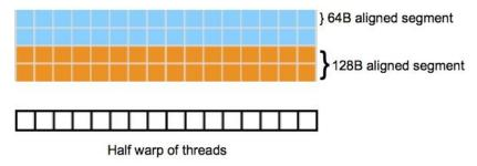
Figure 3.3 Linear memory segments and threads in a half warp
