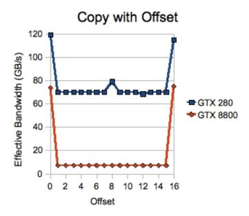
Figure 3.7 Performance of offsetCopy kernel
