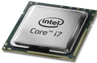
(a) i7 960 (laboDMS) : 4 coeurs (8 threads HT), 3.2 GHz, 12 Go DDR3
